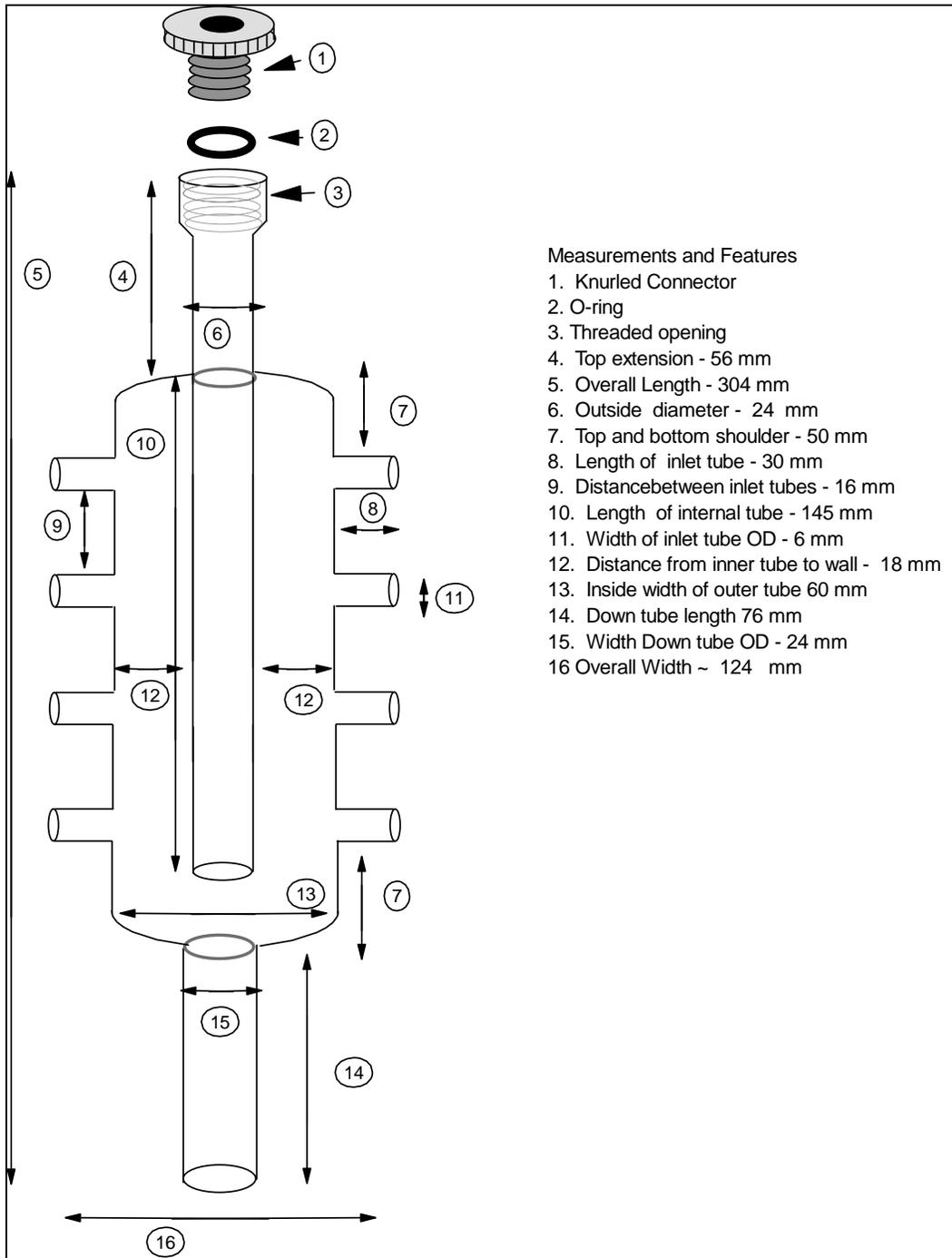
**Figure 4. Specifications for an 'Octopus' Style Manifold**
