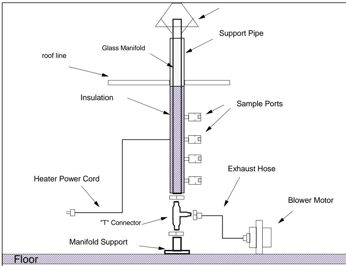
**Figure 5. Example of Vertical Design Manifold**
