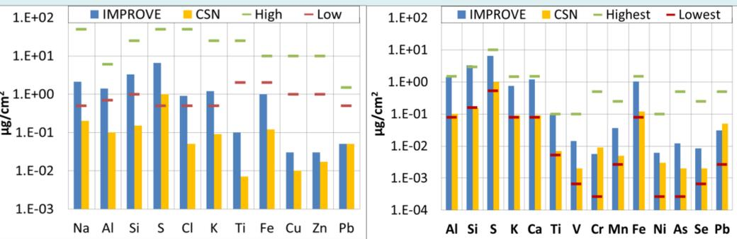
Fig.2. Left) The range of generated SE-RMs (Low and High); Right) ME-RMs (Lowest and Highest) compare to IMPROVE and CSN 90%iles for selected elements.
