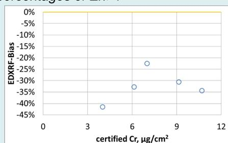
Fig.5. EDXRF bias from certified Cr loadings generated from CrN
