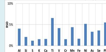
Fig.9. The relative standard deviation (RSD) of a ME-RM weekly analyzed by EDXRF since 2014 ( $n > 200$ ). Low RSD show good stability of generated ME-RMs.
