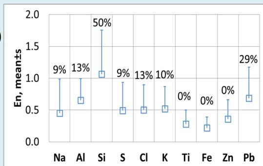
Fig.3. En number of EDXRF vs. certified loadings of SE-RMs. Numbers refer to percentages of  $En > 1$
