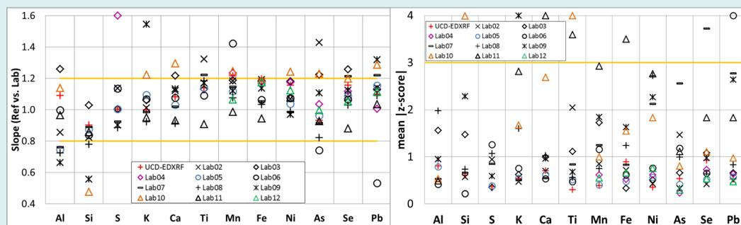
Fig.6. The slopes of reference versus labs for Fig.7. The absolute mean z-score of labs selected elements. Labs 10,11, and 12 are for selected elements. The mean z-score ICP-MS. The slopes higher than 1.6 were higher than 4 were shown at 4 for better resolution
