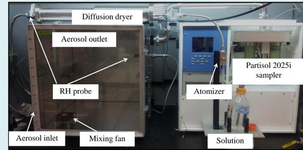
Fig.1. The aerosol generation and sampling system
