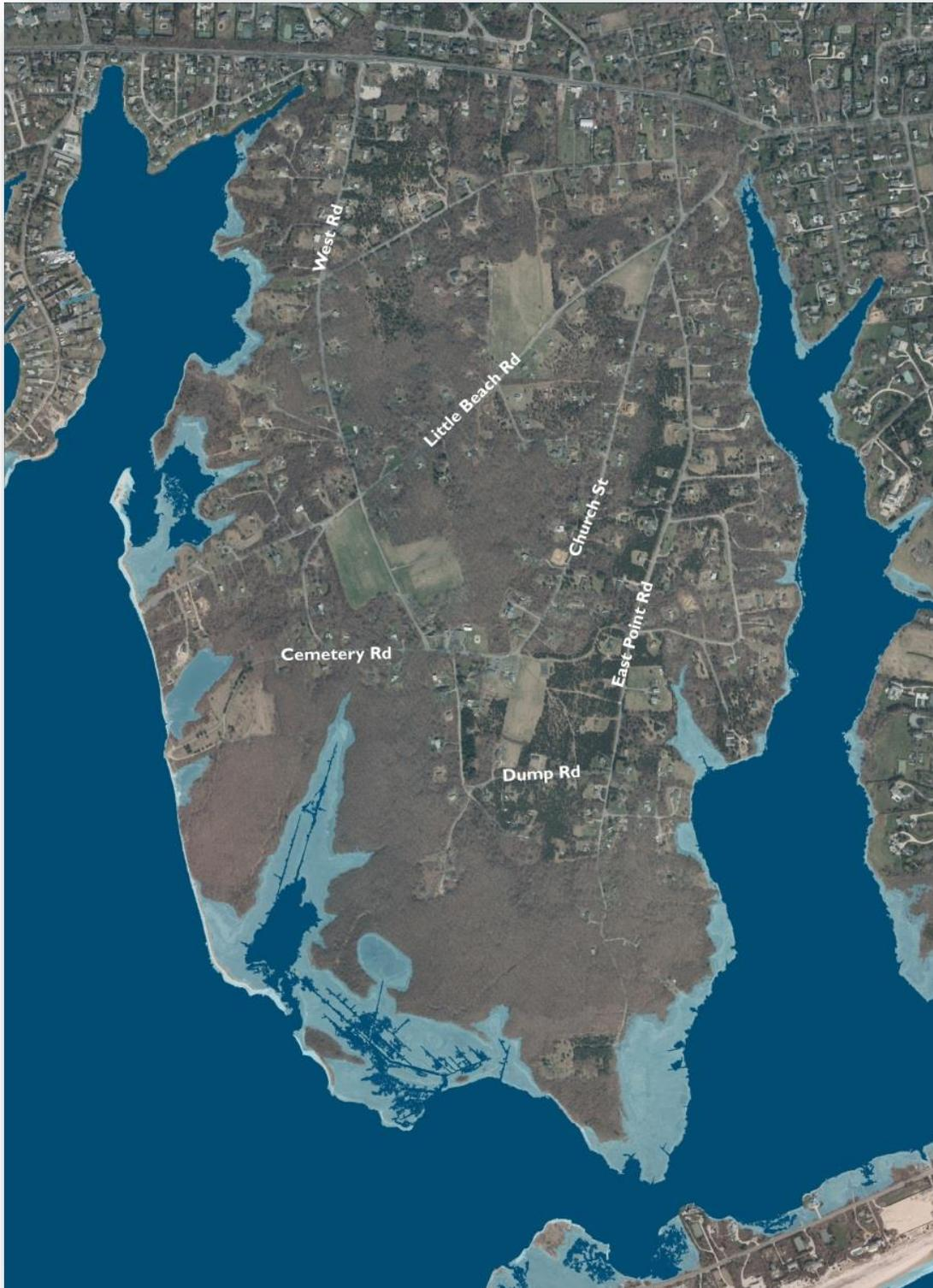
Figure 5. Areas of predicted inundation during mean high water by 2050, assuming that sea level rises 1.5 feet above current levels, consistent with the adjusted “Intermediate-High” NCA global sea level rise scenario.
