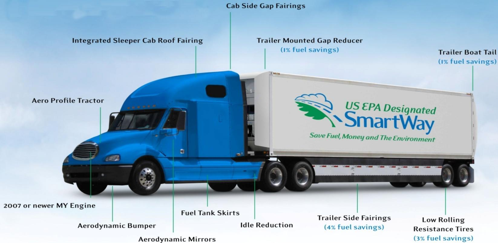
**A SmartWay tractor and trailer annually save 2,000 to 4,000 gallons of fuel and reduce CO<sub>2</sub> emissions by up to 20% as compared to similar trucks on the road. Learn more at [www.epa.gov/smartway](http://www.epa.gov/smartway)**
