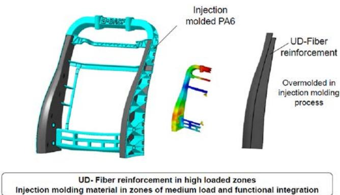
Figure 13. Prototype-Seat Backrest with Over-Molded Tape Reinforcement(Source: BASF)
