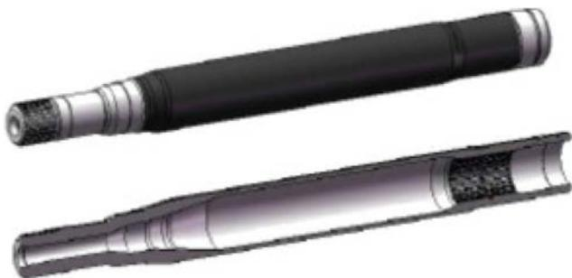
Figure 16. Silverado Vari-Lite® Tube - Axle Half-Shaft(Source: U.S. Manufacturing, Warren, Michigan)
