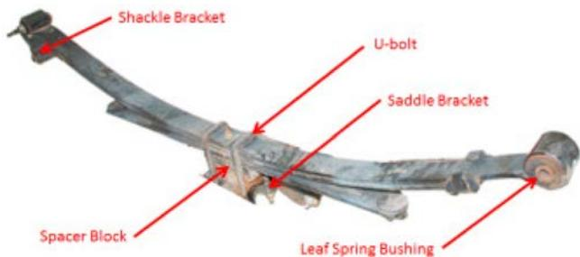
Figure 4. Rear Suspension Subsystem Current Assembly(Source: A2MAC1)
