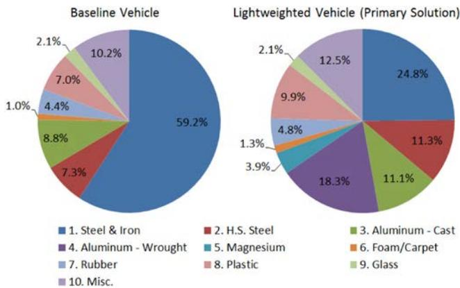
Figure 2. General Material Make-up of 2011 Silverado 1500 Production Vehicle and Lightweighted Vehicle
