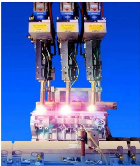
Figure 15. Plasma Transfer Wire Arc (PTWA)(Source:<http://www.geencarcongress.com/2009/05/ptwa-20090529.html>)
