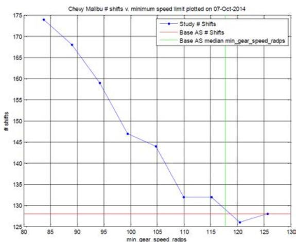
Figure 17. Number of shifts versus min\_gear\_speed\_radps
