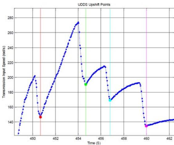
Figure 6. Post-upshift speeds don't have a time delay
