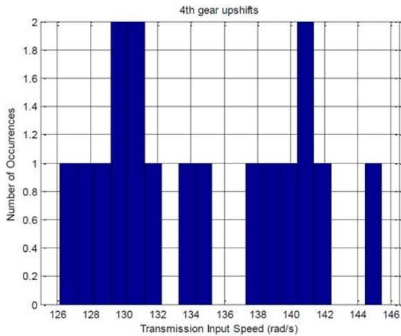
Figure 5. Post-upshift speeds for 4th gear over a UDSS drive cycle
