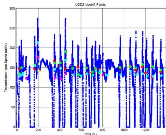
Figure 4. Upshift points over a UDDS drive cycle
