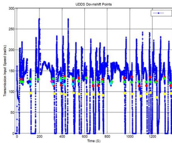
Figure 1. Downshift points over a UDDS drive cycle
