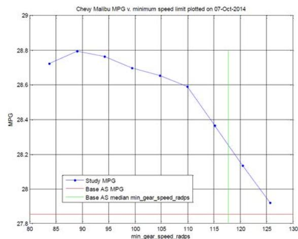
Figure 16. Fuel economy versus min\_gear\_speed\_radps
