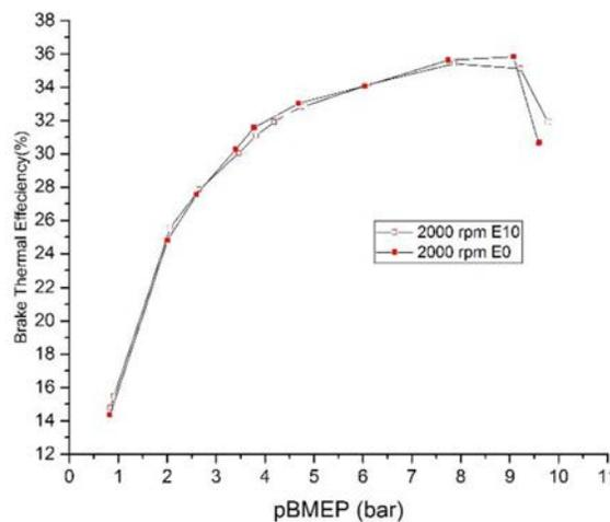
Figure 11. Different Fuels Effect on BTE at 2000 rpm
