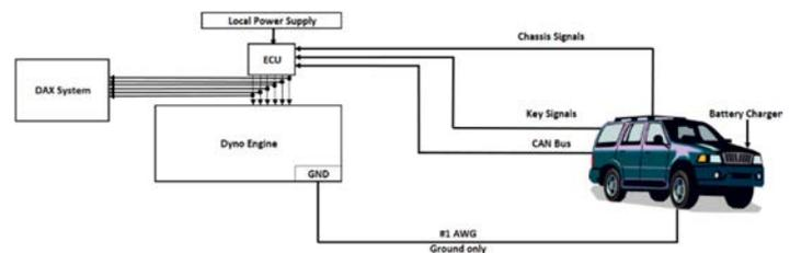
Figure 1. Vehicle and Engine Tethered Wire Harness
