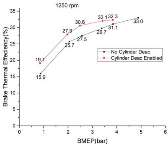
Figure 8. Cylinder Deactivation Effect on BTE at 1250 rpm
