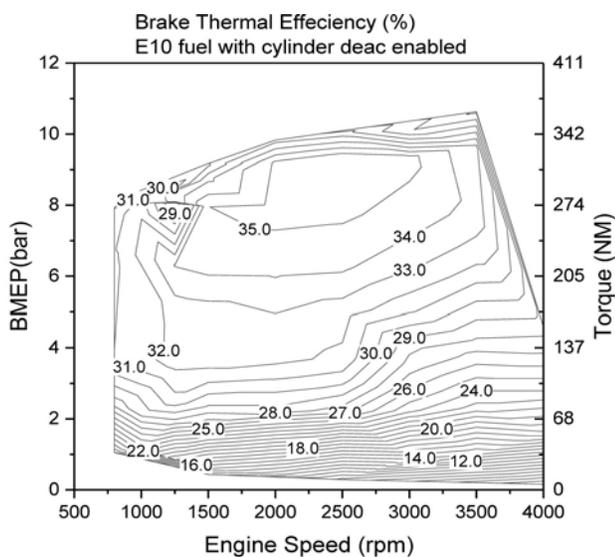
Figure 9. 4.3L Brake Thermal Efficiency, E10 fuel, with Cylinder Deactivation
