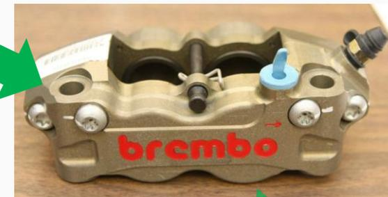
Caliper Housing from cast iron to cast Mg
