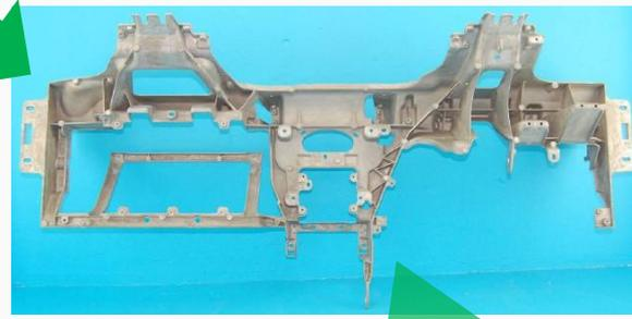
Cross Car Beam from Steel Welded to Die Cast Mg
