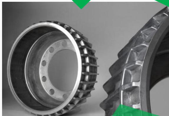
Changing Rear Drum from cast iron to AL, adding cooling fins and cross drilling
