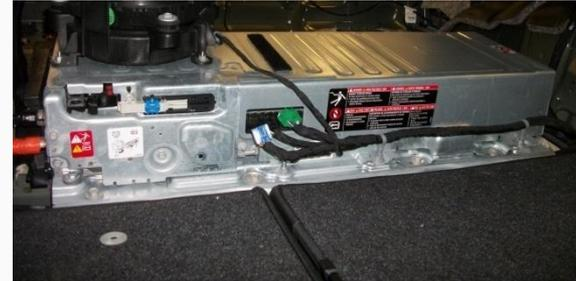
Orange 115v volt cable from starter/generator & black 12v volt cable from main battery, connected to ION battery in trunk to starter/generator in engine compartment
