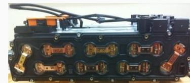
**1 of 2 Battery modules cells exposed**
