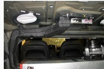
The ION battery fan takes air from the cabin and draws it down through the battery and exhausts into the wheel well
