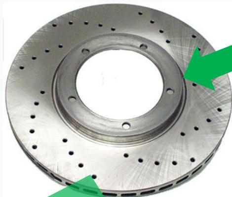
Changing Front Rotor 1 piece iron to 2 piece steel + AL, adding cross drilling, etc
