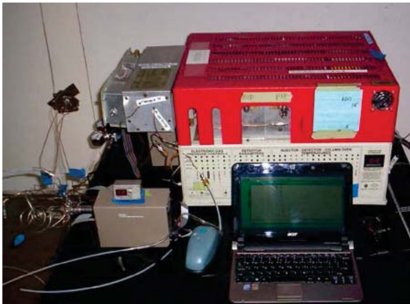
Air monitor EPA researchers use to study vapor intrusion inside a former pre-1920 home.
