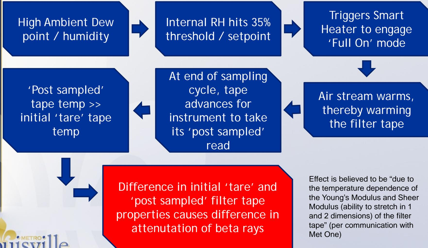
Effect is believed to be “due to the temperature dependence of the Young’s Modulus and Sheer Modulus (ability to stretch in 1 and 2 dimensions) of the filter tape” (per communication with Met One)
