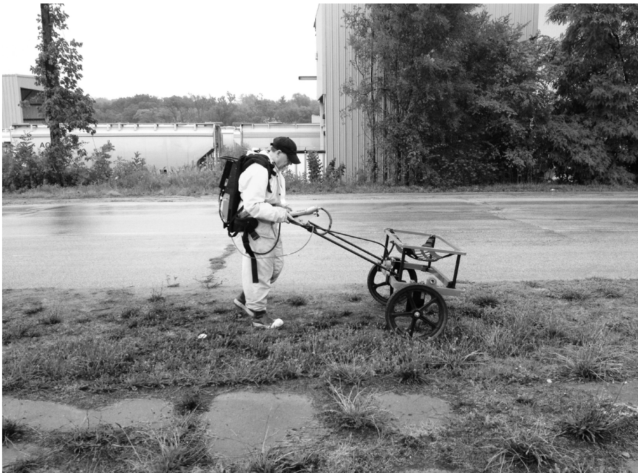
A U.S. EPA employee uses special equipment to check for the presence of underground storage tanks and pipes. U.S. EPA and Illinois EPA are searching for the source of pollution that has contaminated some drinking water wells in the LaSalle County town of Wedron.
