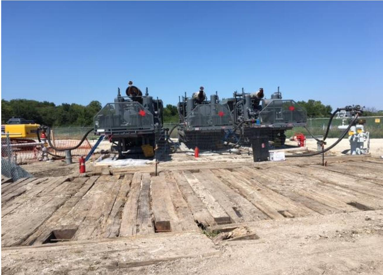
Three 300-hp compressors in parallel operation
