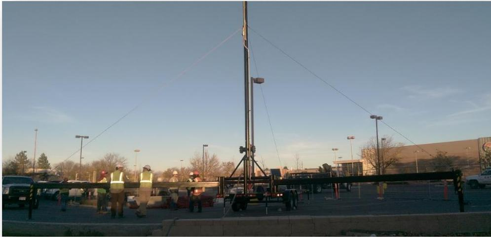
Fully set up 30 foot portable flare
