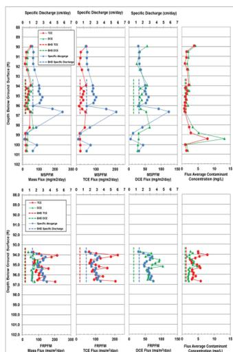
Figure 6. Comparison of FRPFM results with those of a borehole dilution test (BHD) and a modified version of a commercially available passive flux meter (MSPFM).
