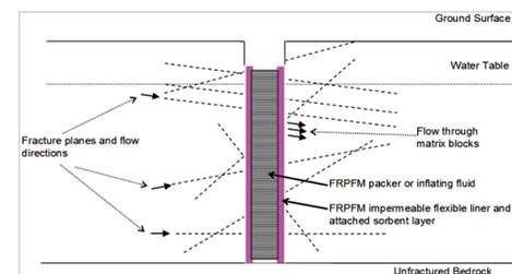
Figure 2. Horizontal cross-section of an FRPFM in a borehole.
