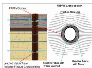
Figure 1. A profile view of an unscreened borehole containing an FRPFM
