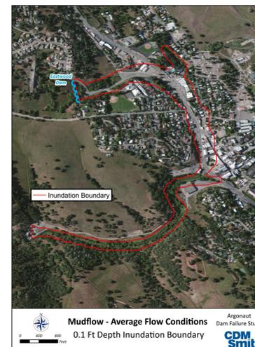
Figure 4: Inundation Boundary, Argonaut Dam Failure Study
