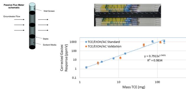
The lower right graphic above shows results from experiments conducted to investigate the use of Gastec tubes (upper right) as a field-based analysis method for passive flux meters. Passive flux meters are used to measure contaminant flux, and a conceptual depiction is shown in the left graphic above.
