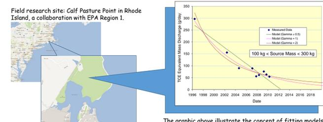
The graphic above illustrates the concept of fitting models to mass discharge measurements to predict source behavior, and to better link characterization, prediction, and decision making.
