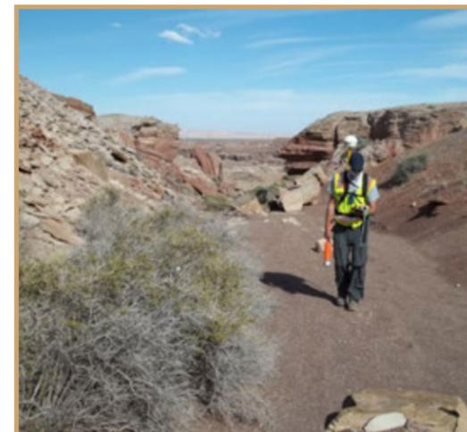
In this picture, a worker uses special equipment to find radiation and protect himself while he works. Knowing where these mines are and their level of radiation will help to get them cleaned up.
