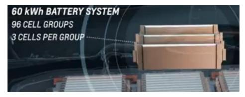
Trend toward flat, floor mounted packs using large, low-profile cells
