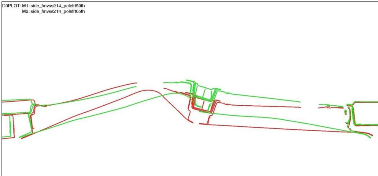
*Figure 4.5.4.3.1.a: 5<sup>th</sup> percentile female vs. 50<sup>th</sup> percentile male front door intrusion comparison*
