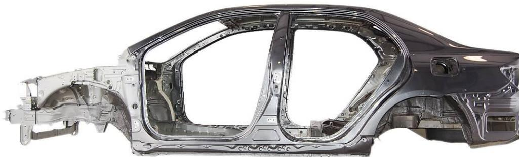
*Figure 4.5.8.1.7.b: Toyota Corolla body-in-white structure*
