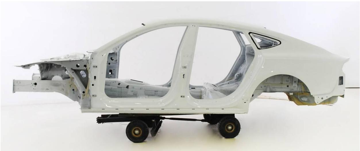
*Figure 4.5.8.1.7.d: Audi A7 body-in-white-structure*
