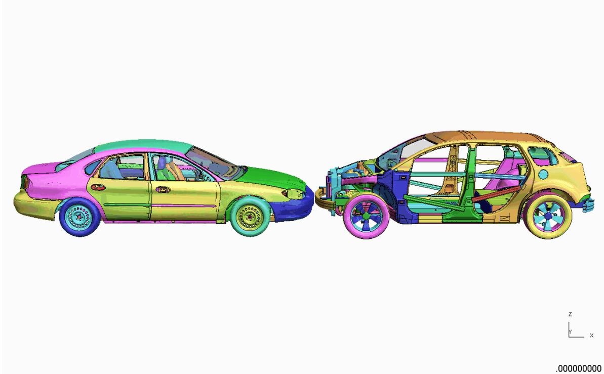
Figure 4.4.9.b: Phase 2 HD vehicle to Ford Taurus crash simulation setup – side view
