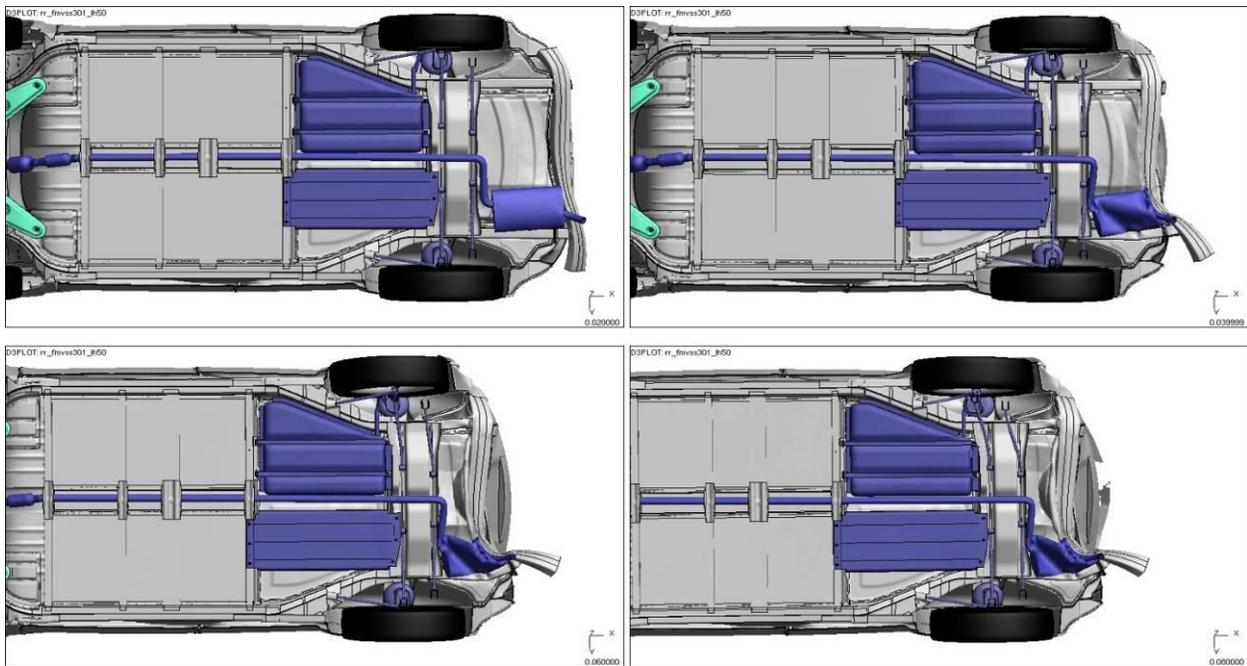
Figure 4.5.4.5.d: Vehicle Deformation (@ 0ms/40ms/80ms/120ms) after rear impact
