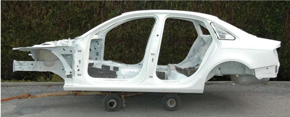
*Figure 4.5.8.1.7.c: Audi A4 body-in-white structure*
