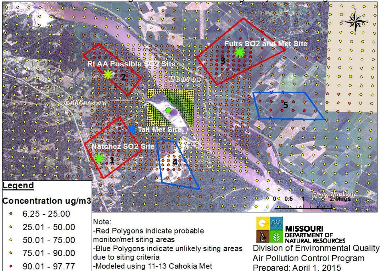
Figure 2. High impact areas and probable SO<sub>2</sub>/Meteorological (Met) station siting areas based on dispersion modeling and siting visit
