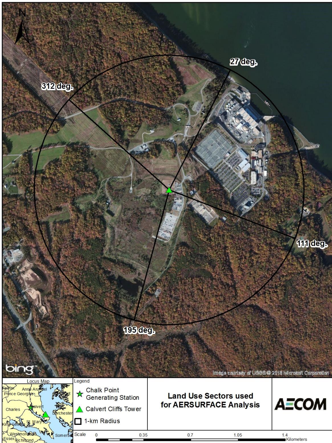
Figure 3-5 Sectors Used for Surface Characteristics at Calvert Cliffs Meteorological Tower
