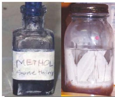
Chemicals that are not correctly and clearly labeled, as shown in the photos above, should be disposed of properly. Products used in schools should have an MSDS, be stored in their original containers, and be correctly and clearly labeled.
