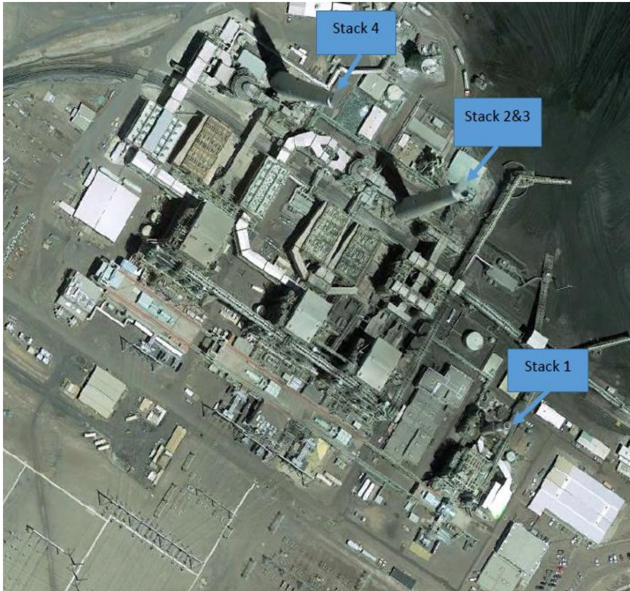
Figure 5-1 Modeled Emission Sources in APS-Cholla Power Plant
