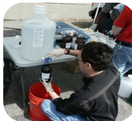
**Figure 2-1. Sub-sampling from a Large Volume Container**
