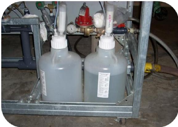
**Figure 2-3. OWQM Station with Sample Collection Containers**
