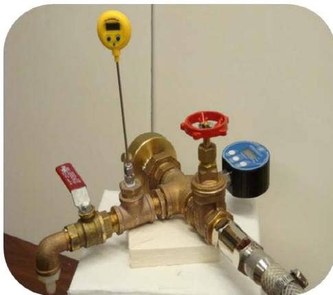
**Figure 2-2. Hydrant Sampler**
