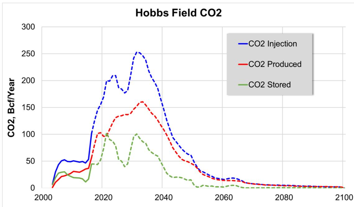
Figure 1 – Hobbs Field Historic and Forecast CO<sub>2</sub> Injection, Production, and Storage 2003-2100
