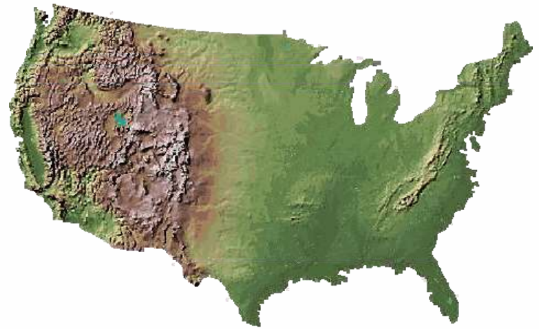
A shaded-relief representation of the conterminous United States portion of the National Elevation Dataset (NED). Elevation is portrayed as of range of colors, from dark green for low elevations to white for high elevations (USGS, 1999—S05140301)
