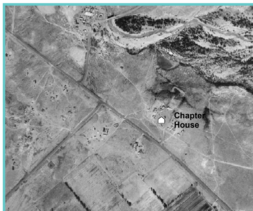
USGS Digital Orthophoto Quarter Quadrangles (DOQQ) are 1-meter ground resolution images that were used by NRCS to create county-wide mosaics. Like the DRGs, the DOQQ mosaics were compressed to a ratio of about 1:20. The example above shows the community of Round Rock (same area as shown left) and illustrates that orthophotos combine the image characteristics of a photograph with the geometric qualities of a map. These county-wide DOQQ mosaics (photos taken in 1997 and 1998) are provided for the entire Navajo Nation in MrSID compressed format.
