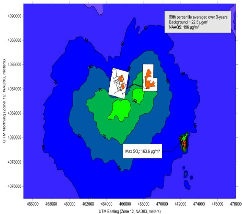
**Figure 2. Navajo Generating Station 1-Hour  $\text{SO}_2$  Air Dispersion Modeling Results**
