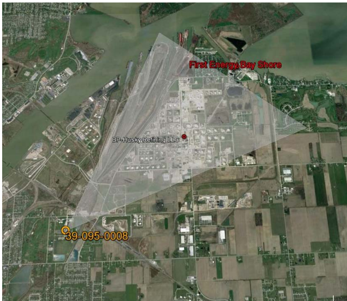
Figure 4: Monitor and source locations for the Bay Shore and BP Husky source area, with 22° - 67° wind sector.
