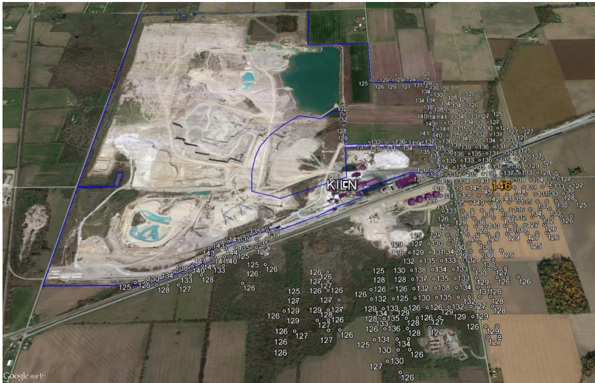
Figure 5: Maximum SO 2 impacts, Carmeuse Lime Maple Grove facility, 2012-2014. Concentrations in µg/m 3 , including background.
