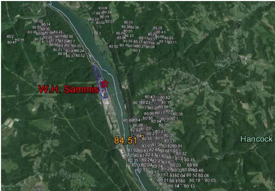
Figure 4: Maximum SO 2 impacts, First Energy W.H. Sammis facility, 2012-2014. Concentrations are shown in µg/m 3 including background.
