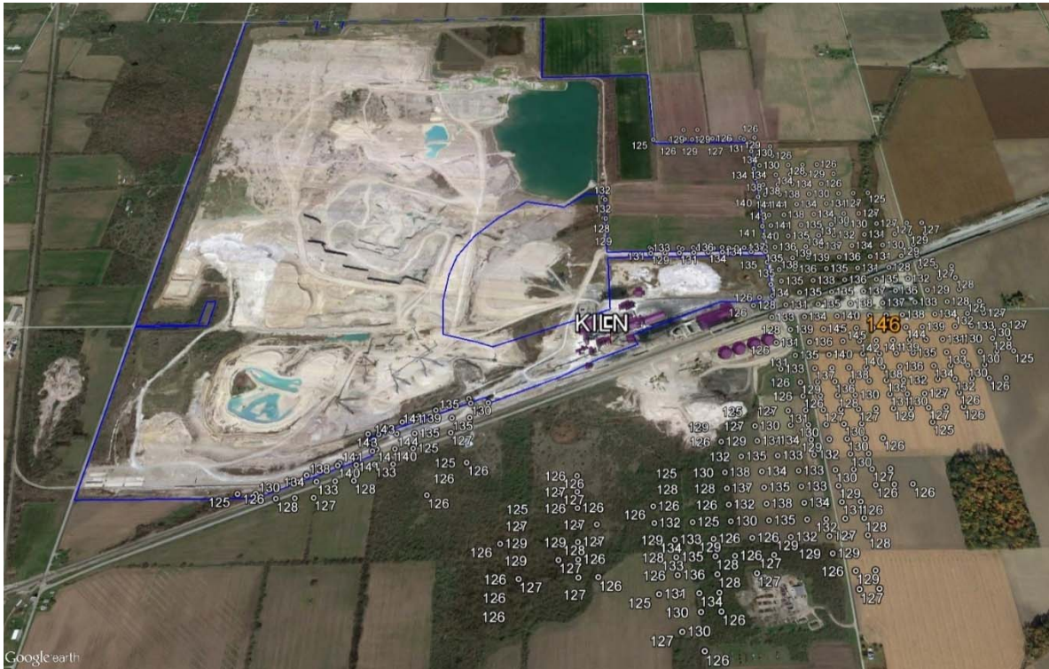
Figure 6: Maximum SO 2 impacts, Carmeuse Lime Maple Grove facility, 2012-2014. Concentrations are shown in \mu\text{g}/\text{m}^3 including background.
