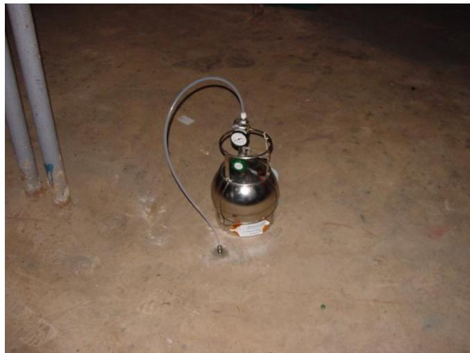
An example of an individual summa canister of the type used to collect sub-slab vapor samples.
