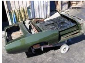
Because only steel (plus copper and brass) can safely go into the dipping tank, the vehicl
