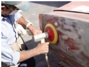
Sanding with 80-grit paper on a rotary or dual-action sander is a good way to attack the t
