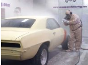
Not inclined to spend days sanding your ride? Media blasting strips automotive paint quick
