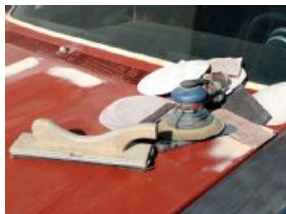
Tools of the sanding trade, found at Paint n Place in Placentia, California: Sanding board
