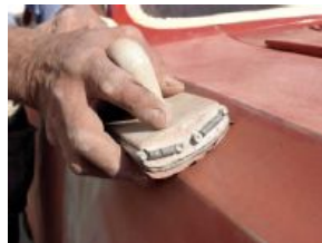
Not all sanding boards are flat. Note the curvature along the bottom of this board and how
