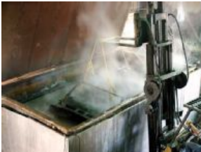
Tank dipping, as seen here at Strip Clean, is chemical stripping taken to the extreme. The
