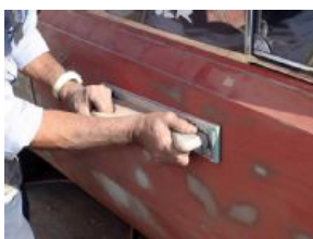
Using a sanding board on broad, flat surfaces (such as this GTO door) helps the sandpaper
