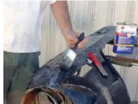
Many do-it-yourselfers prefer chemical stripping to sanding because it's faster and requir
