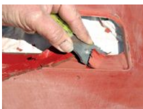
Believe it or not, a razor blade can be just as effective as -- if not faster than -- sand
