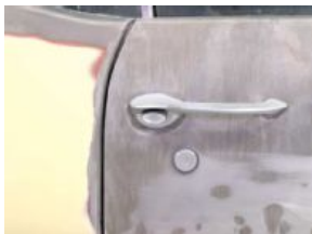
Baking soda, which is used by Anacapa, is one of the less-aggressive blasting media. It'll
