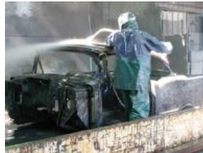
After the car soaks in the tank for several hours, it's pulled out and hosed down with w at
