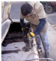
Media blasting is messy. Because the Camaro's taillights were removed before blasting, the
