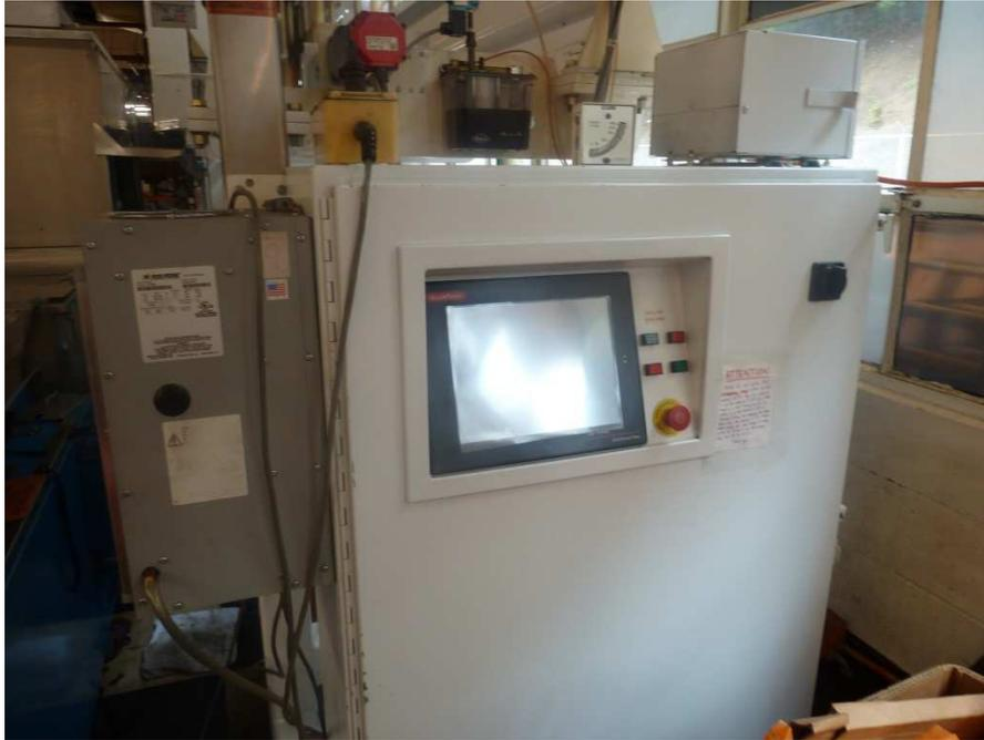
Greco Robot Actuated Degreasing System – Programmable Logic Control (PLC)
