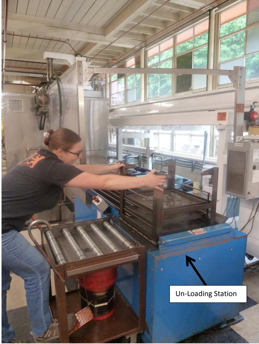
Greco Robot Actuated Degreasing System - Rear
