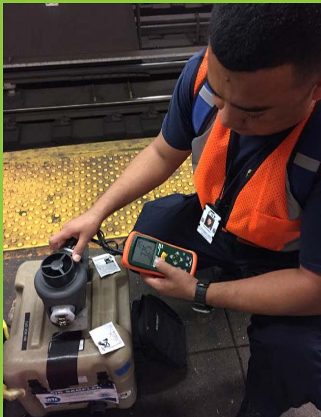
Verifying the flow rate of the dry filter unit sampler
