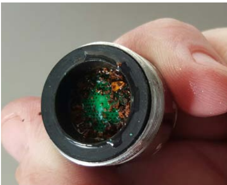
Faucet aerator residue sampled for metals
