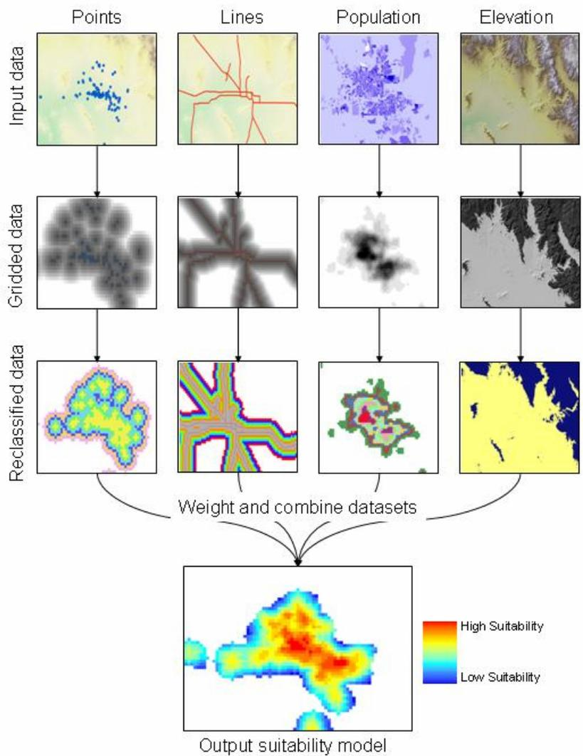
**Figure 2.** Conceptual approach for building a suitability model.
