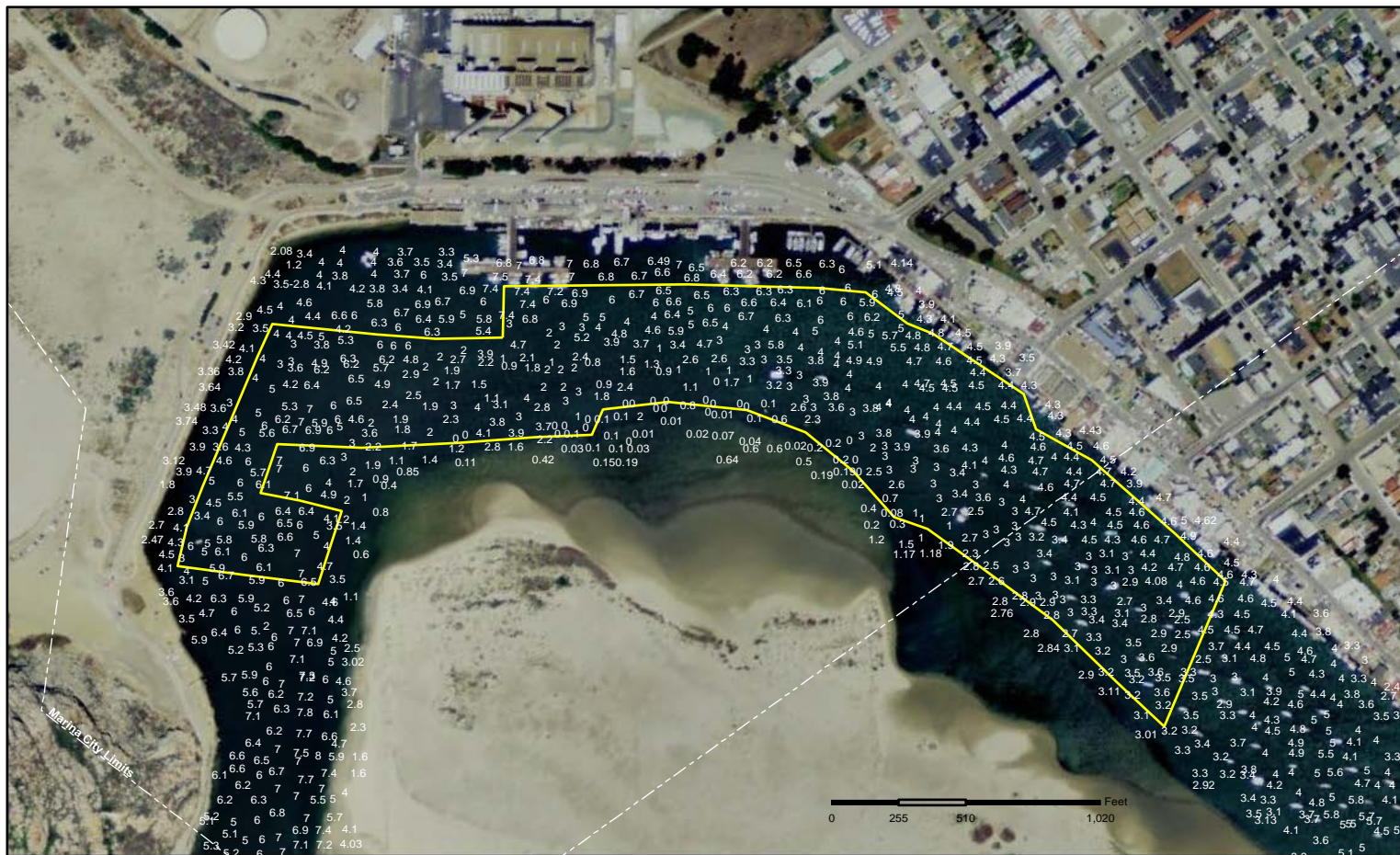
Plan View of Existing Bathymetry within the Proposed Dredging Boundaries
