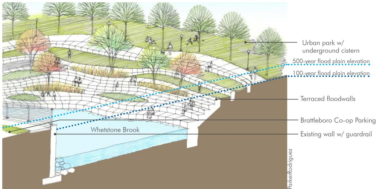
FIGURE 26. Normal Brook Elevation
