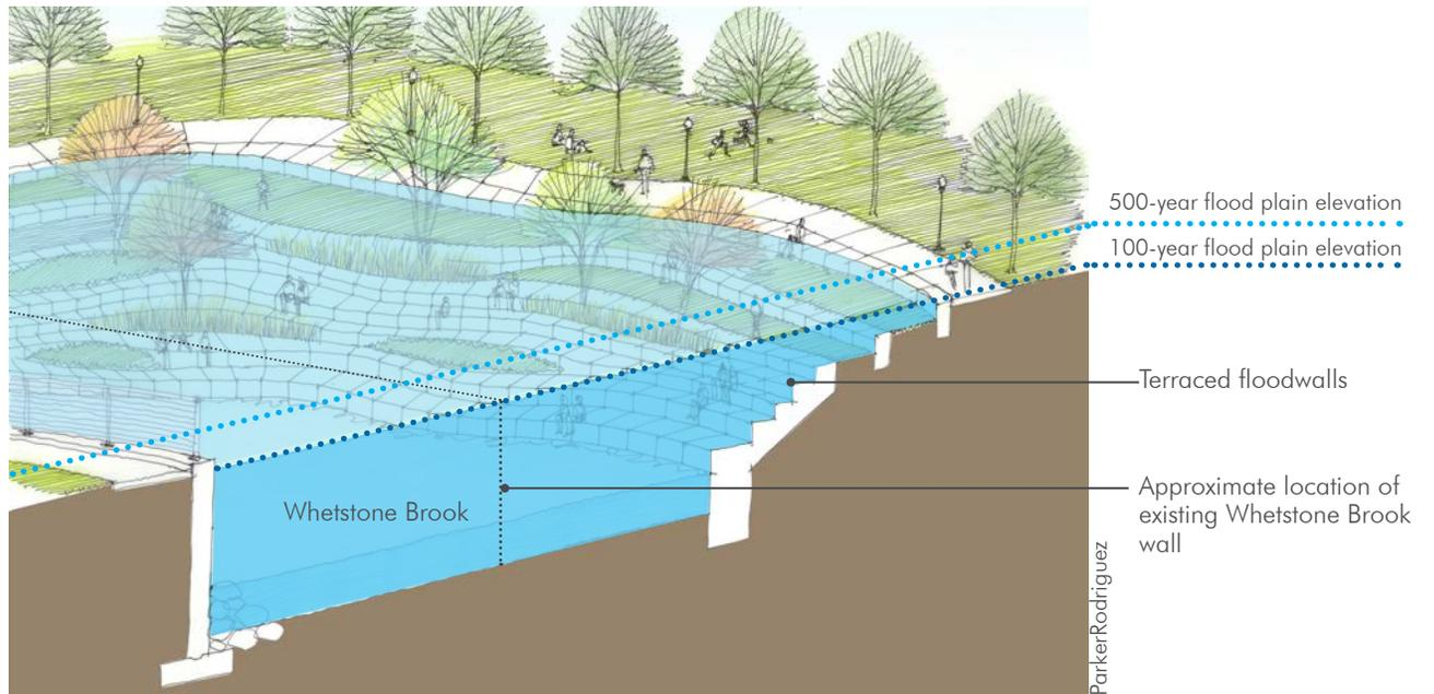
FIGURE 28. Proposed conditions flood plain elevation
