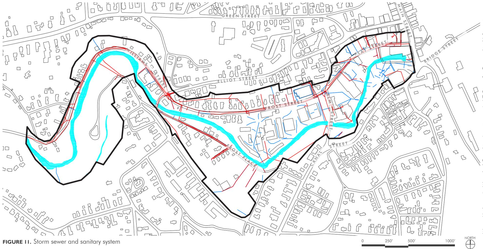
FIGURE 11. Storm sewer and sanitary system
