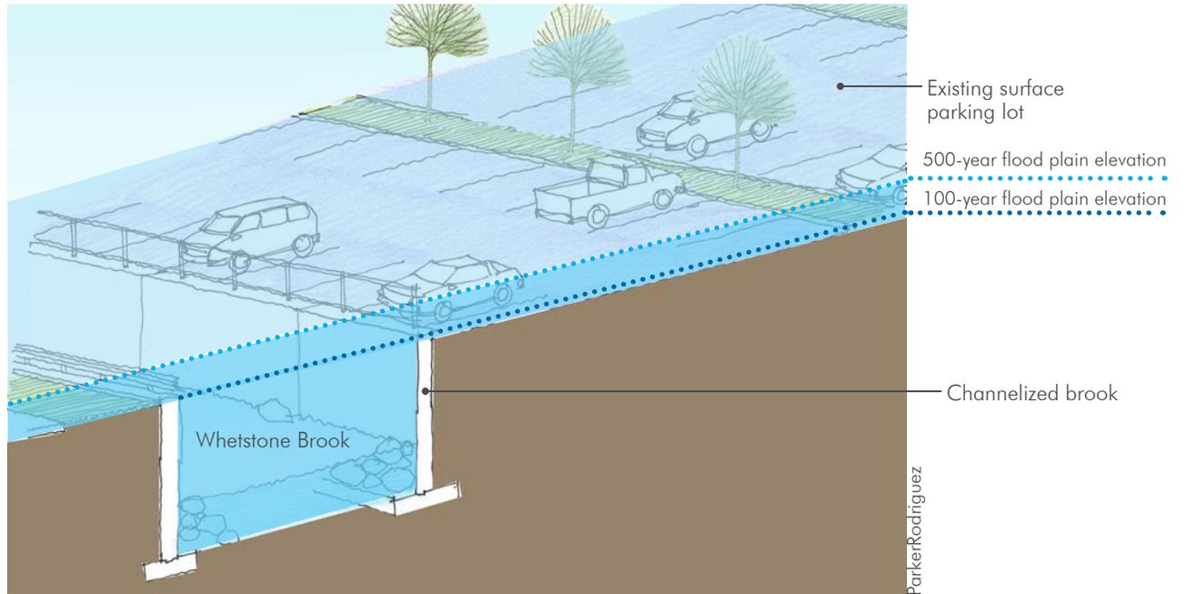
FIGURE 27. Existing conditions flood plain elevation
