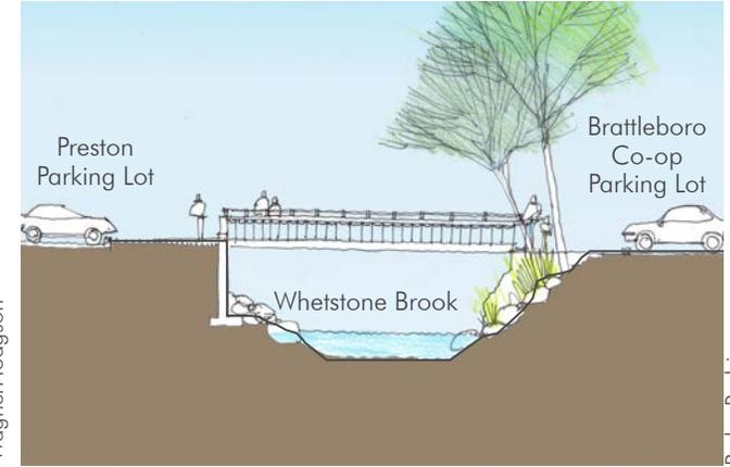
FIGURE 14. Existing section enlargement of channelized brook
