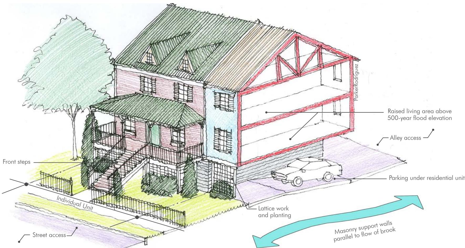
**FIGURE 49.** Proposed resilient housing configuration
