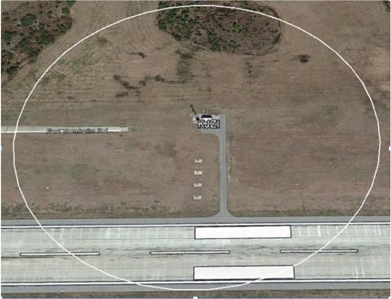
Figure 30 Anemometer site at KJZI with 100m radius circle
