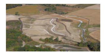
Remedies included relocating a stretch of Glade Creek, excavating sediment from a downstream stretch and Construction of Creosote Recovery Trenches (photo circa 2005)
