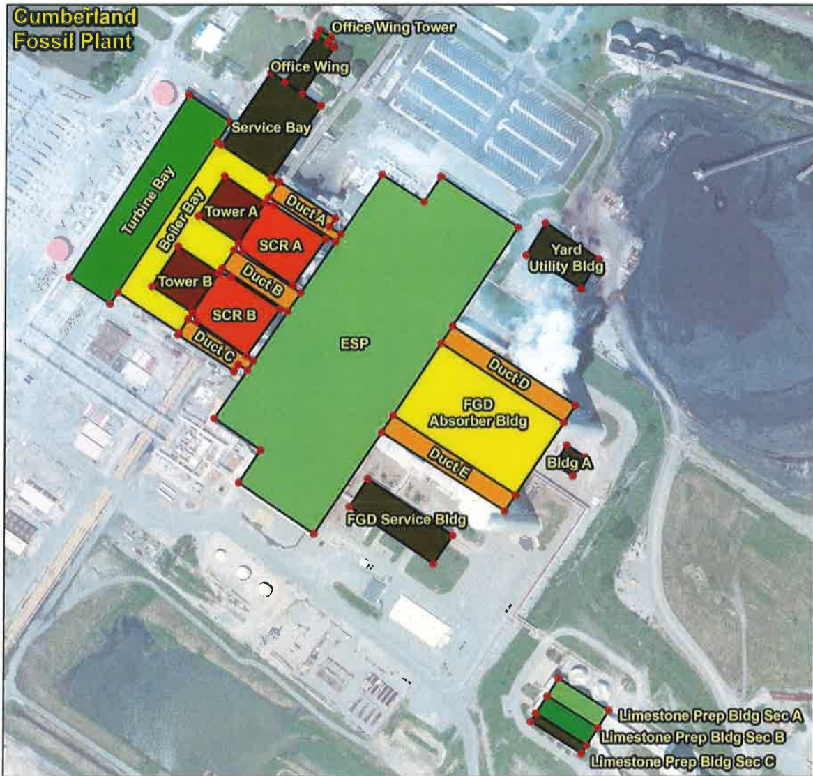
Figure 3 Building Locations for Stack Downwash Analysis
