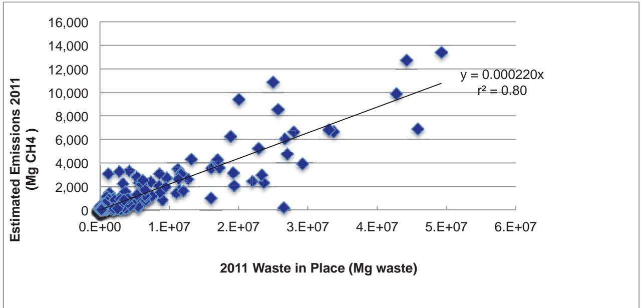
Fig. 2. (a) ABOVE: Relationship between estimated 2011 site-specific landfill CH<sub>4</sub> emissions using IPCC (2006) and WIP for 371 California landfills. (b) BELOW: Same relationship including the large Puente Hills Landfill [N=372]. Data from California Air Resources Board [ARB] (Hunsaker, 2012). NOTE: Predicted emissions from WIP using regression coefficients are 190-220 Mg CH<sub>4</sub>/million Mg WIP. Figure reprinted from Bogner et al., 2016.
