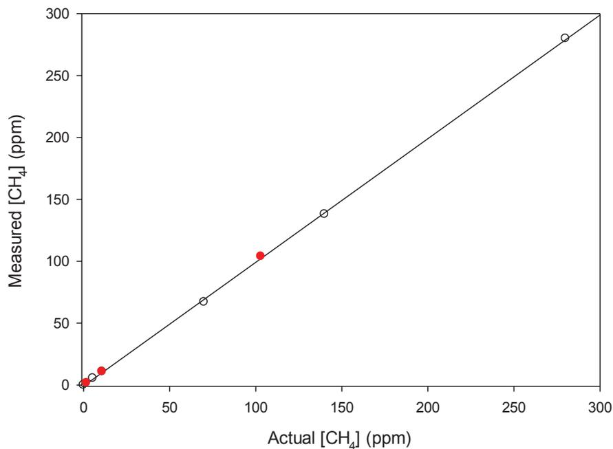
**Figure 3.2. Calibration curves obtained for the methane analyser. Open circles correspond to points made using gas mixtures generated with a gas diluter. Red circles represent a multipoint calibration made using reference gases several months later.**
