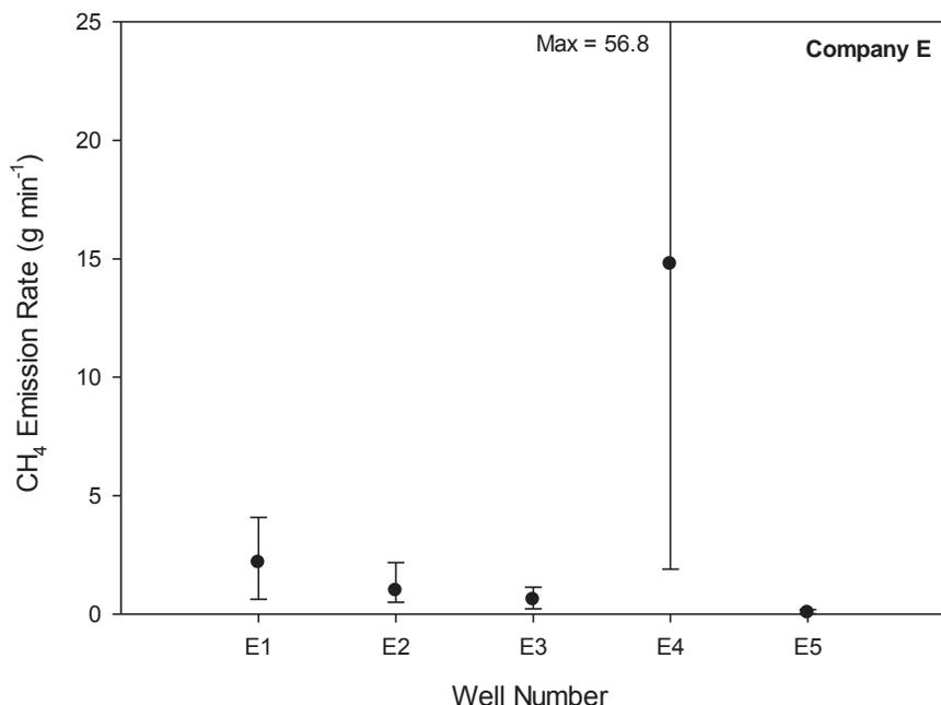
Figure 4.11. . Total CH<sub>4</sub> emission rates estimated at Company E's well sites using the traversing method.
