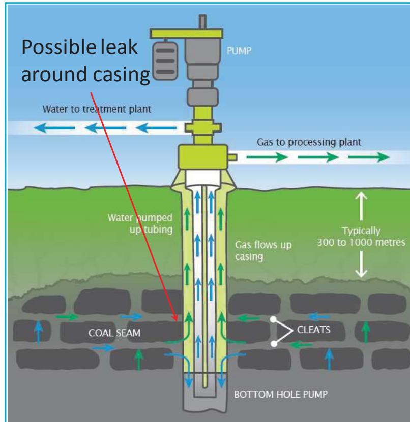
Figure 4.12. Schematic representation of a CSG well showing a possible route for CH<sub>4</sub> leaking outside a casing.
