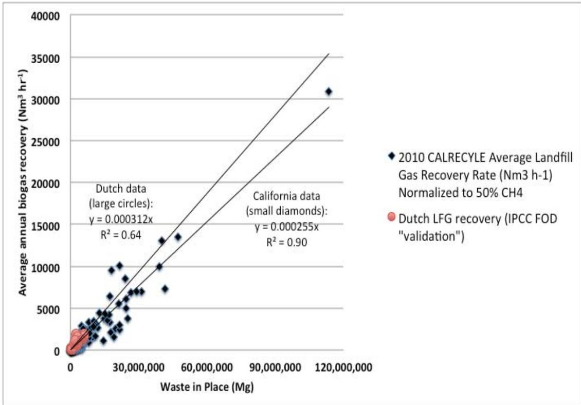
Fig. 1. Comparison between WIP and average biogas recovery rate for: (a) 2010 data from Calrecycles for 129 California sites (Walker et al., 2012): *blue diamonds*; and (b) IPCC FOD model field validation data from 9 Dutch landfills (1986-1993) (Oonk & Boom, 1995): *red circles*. Figure reprinted from Bogner et al., 2016.
