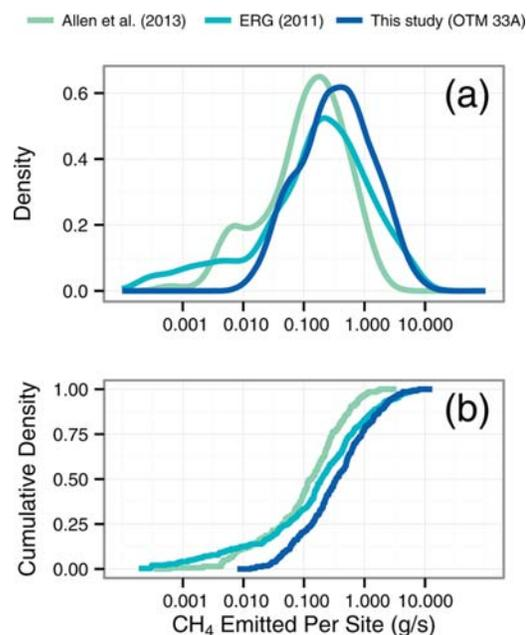
**Figure 4.** Density (a) and cumulative density (b) of measurements of  $\text{CH}_4$  emission rates (g/s) from this study (OTM 33A), Allen et al.,<sup>16</sup> and ERG.<sup>15</sup> Note the logarithmic x-axis.
