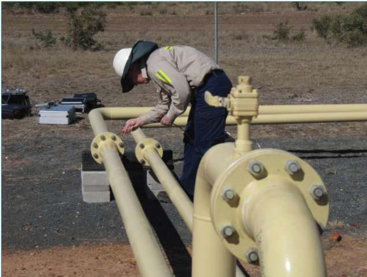
Figure 3.4. Locating equipment leaks at a CSG well pad.
