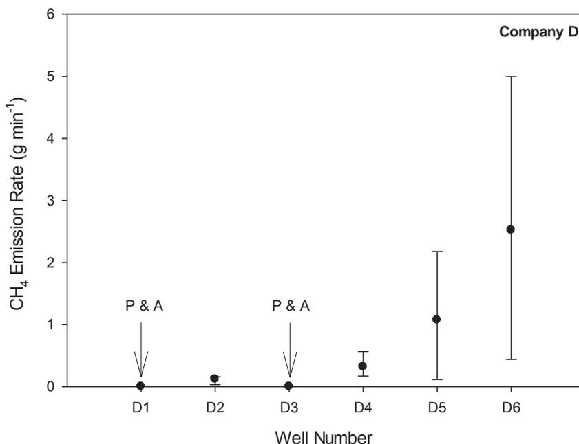
Figure 4.9. Total CH<sub>4</sub> emission rates estimated at Company D's well sites using the traversing method.
