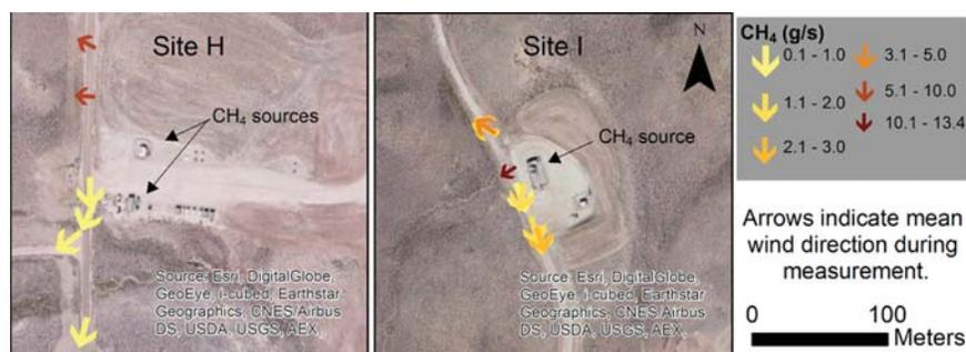
**Figure 2.** Map of repeated measurements at sites H and I. The directions of the colored arrows indicate mean wind directions and the locations indicate the locations of the mobile platform during the measurement.
