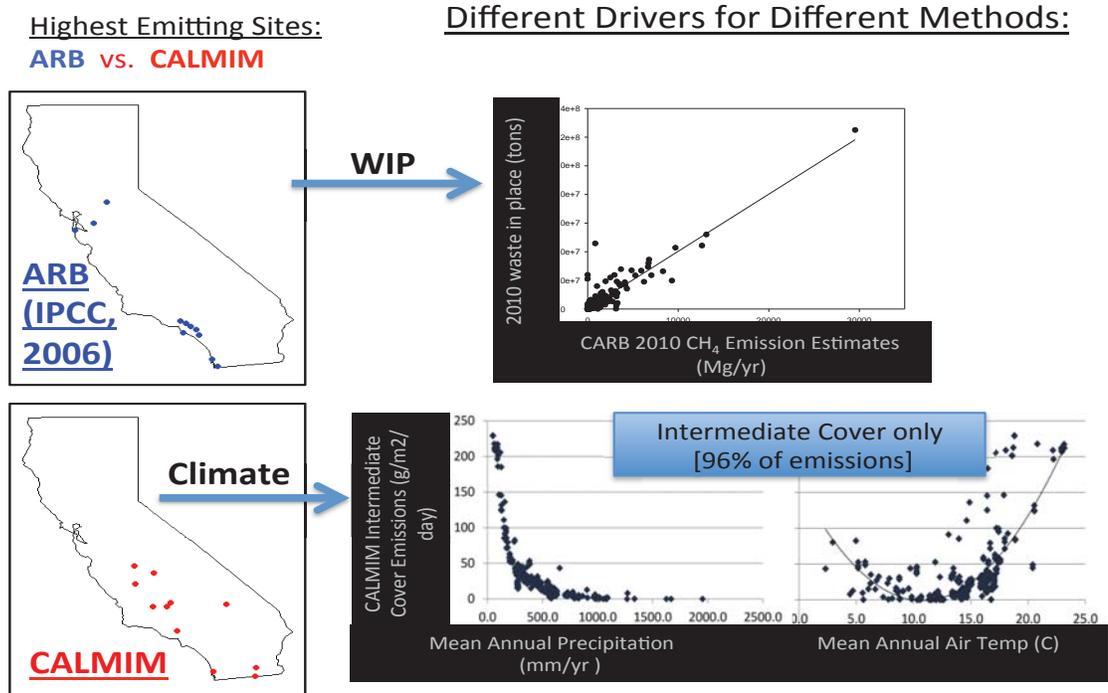
Fig. 5. Comparison of major dependencies for estimated California landfill CH<sub>4</sub> emissions using:
