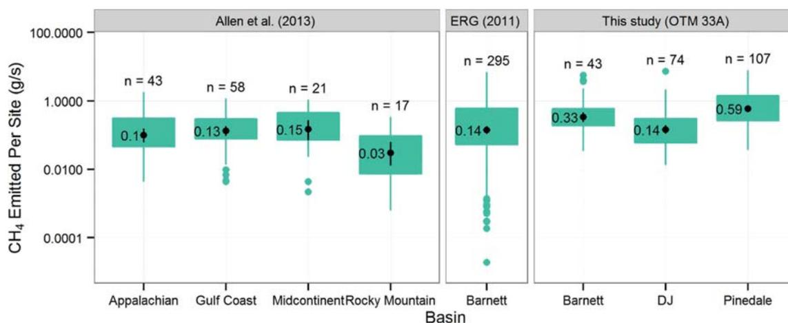
**Figure 3.** Comparison of measured  $\text{CH}_4$  emissions per pad (g/s) from Allen et al.,<sup>16</sup> ERG,<sup>15</sup> and OTM 33A by basin. Boxes represent the 1st and 3rd quartiles of the data, while whiskers extend to the largest measurement that is within 1.5 times the interquartile range (IQR). Means and 95% CIs are shown in black and were calculated using a nonparametric bootstrap.
