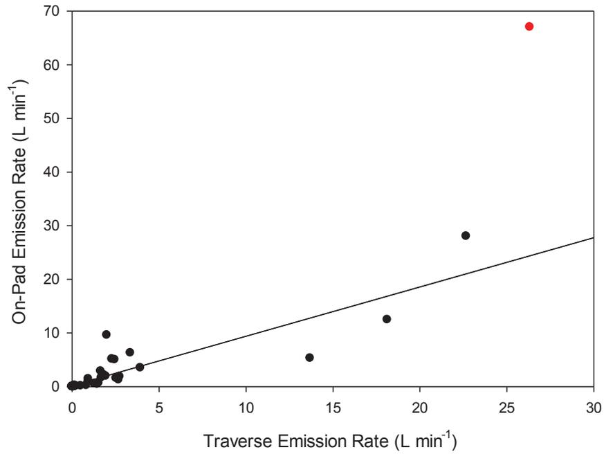
**Figure 4.4. Correlation of total CH<sub>4</sub> emissions determined by traverses with on-pad measurements**
