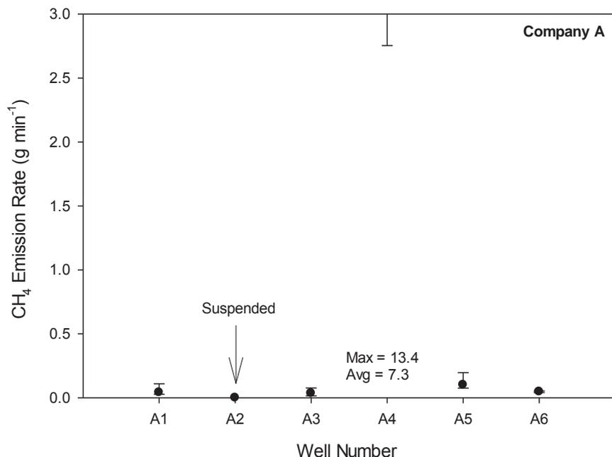
**Figure 4.5. Total CH<sub>4</sub> emission rates estimated at Company A's well sites using the traversing method.**
