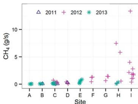
**Figure 1.** CH<sub>4</sub> emission rates (g/s) measured at repeated sites in Pinedale, WY by year.
