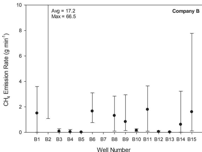
**Figure 4.6. Total CH<sub>4</sub> emission rates estimated at Company B's well sites using the traversing method.**
