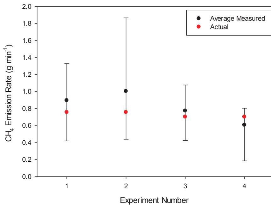
**Figure 4.1. Summary of the controlled release experiments showing the CH<sub>4</sub> release rate determined by plume traversing and the actual release rate. Downwind distances were: Exp No 1 = 20 m; Exp No 2 = 30 m; Exp No 3 = 15 m; Exp No 4 = 30 m. The error bars represent the range of emission rates measured during each set of six traverses.**
