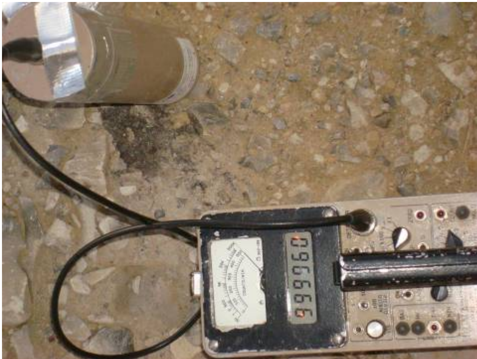
Photo 4. Ruby No. 3 Mine site, very high gamma radiation emitting from black uranium ore
