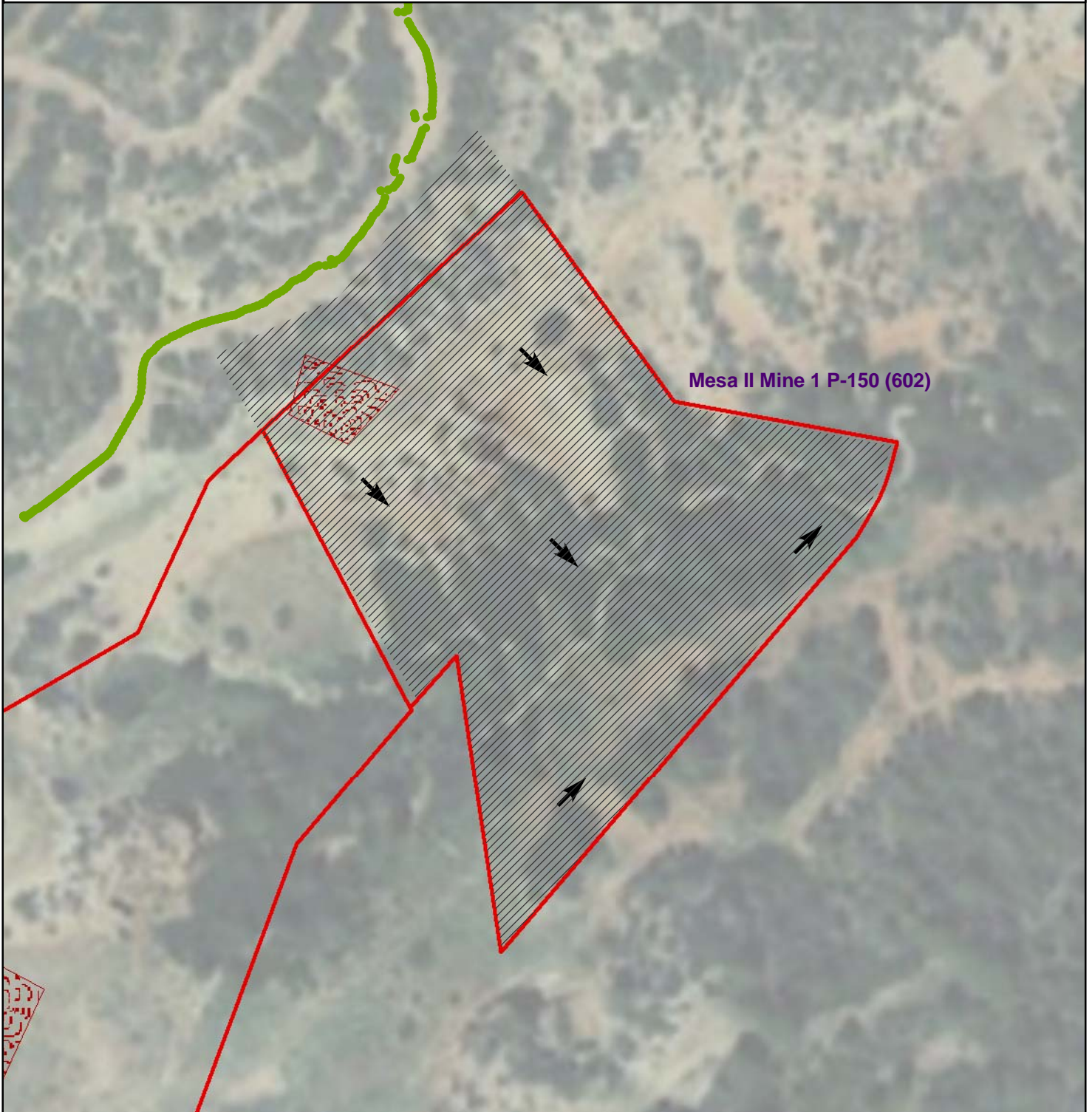
Figure 1 - Gamma Radiation Measurements, Above Two Times Background Mesa II Mine 1 P-150 (602) Cove Chapter, Navajo Nation, Arizona
