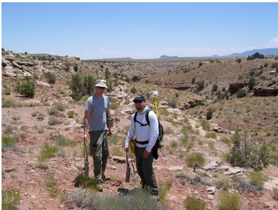
**Photo 4: WESTON used a combination sodium-iodide scintillation detector and a GPS unit (right). A stand-alone scintillation detector also was used (left).**
