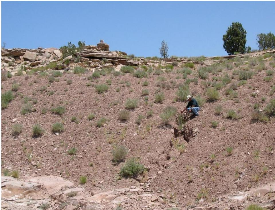
**Photo 2: WESTON detected gamma measurements in excess of 100,000 cpm in an eroded section of the cap at the VCA Plot 7 Mines.**
