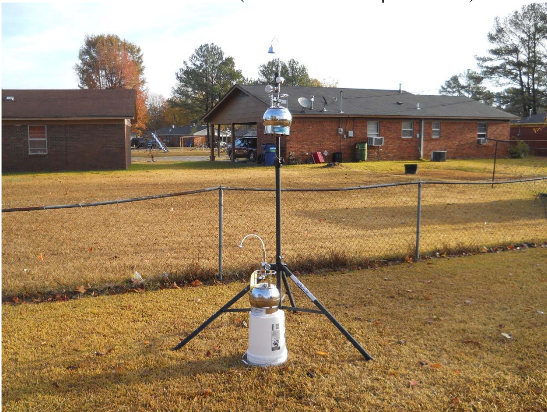
Image 6 – RELOCATED Sample station GM11 - West Ambient Air Monitoring Station facing east DSCN4556 – Taken 11/30/2016 08:01 (co-located Atlas sample on bucket)
