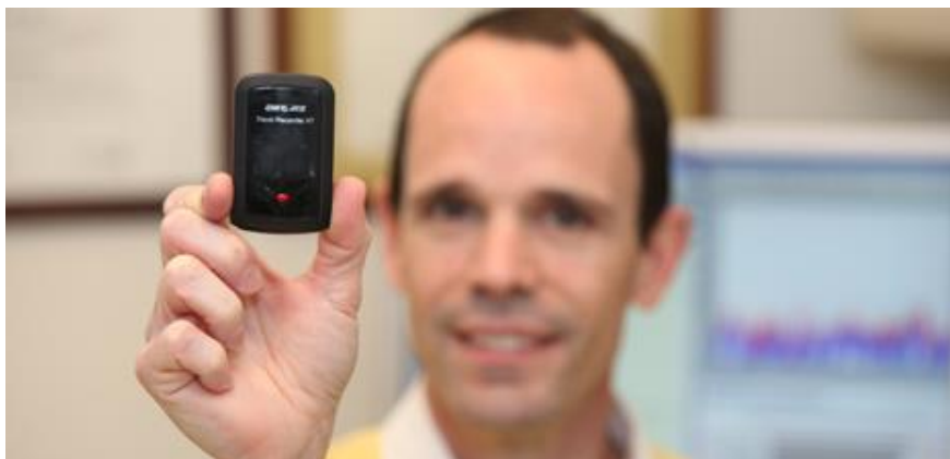
GPS data loggers like this one collect information on a person's location and speed for input into MicroTrac.
