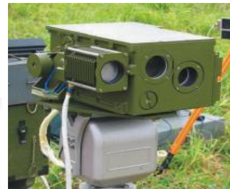
Board passive distant gas meter for methane concentration
