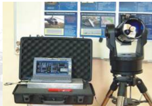
Laser system of the methane spatial concentration
