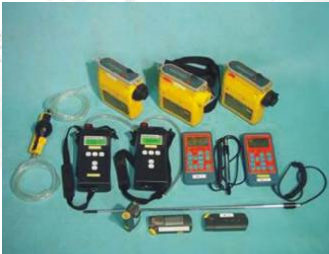
Leakage detectors, methane concentration meters
