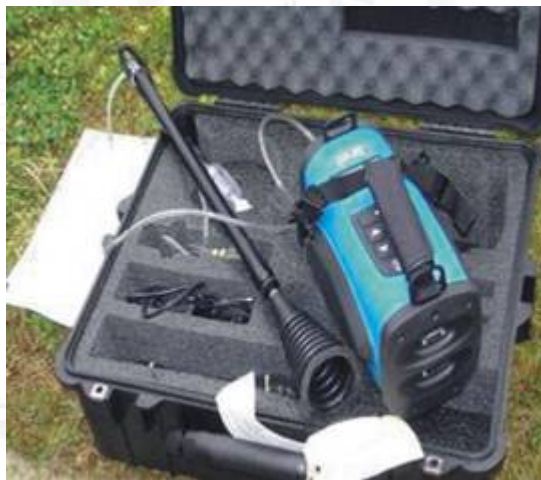
Volumetric emissions measuring and detection device
