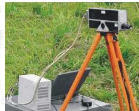
DGA of methane concentration based on an IrDA sound and optical spectrometer and projector
