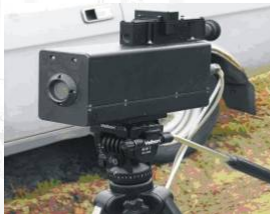
Portable passive gas analyzer for methane
