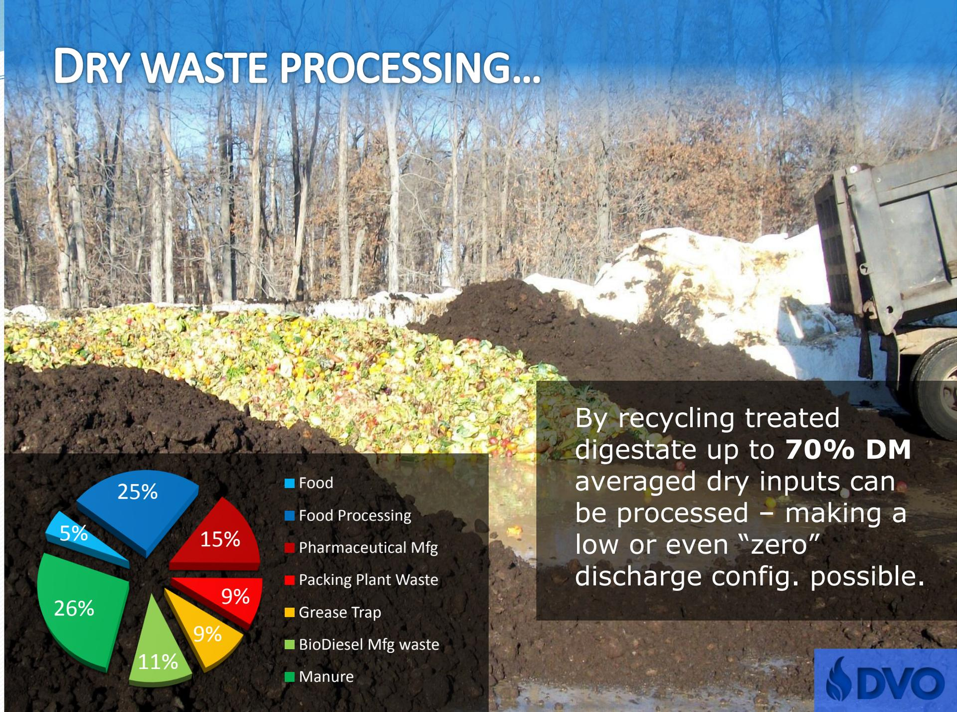
By recycling treated digestate up to **70% DM** averaged dry inputs can be processed – making a low or even “zero” discharge config. possible.
