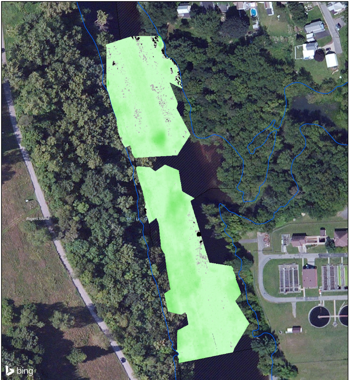
Figure A7-2b. CU-2 Bathymetric Comparison 2009 Cap Reference Survey vs. 2014 Five-Year Tier 1 Survey
