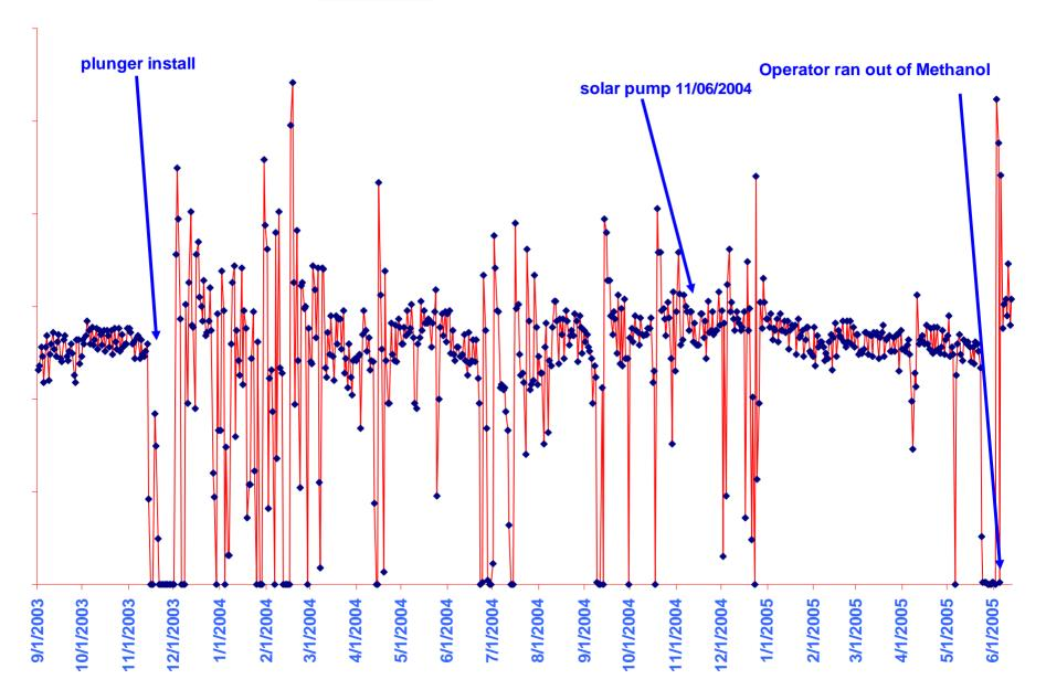
From 8/2003 this well had a Texsteam pump with a rate of 8 gls/day, until 12/14/2004 when the solar pump was installed at a rate of 2.5 gls/day
